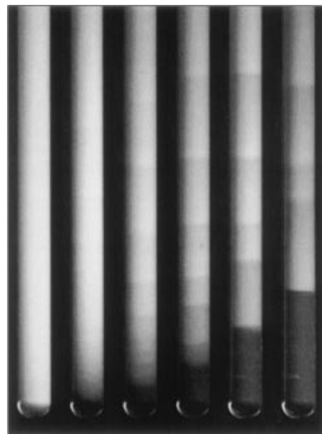
FIG. 1. Images of a 12 mm inner diameter vertical tube of emulsion evolving over time. Visible intensity steps in the rightmost photographs indicate steps in decane droplet concentration, with brighter regions having higher concentration. From left to right, photos were taken after 0, 51, 73, 100, 137, and 175 h of creaming.
